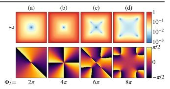
FIG. 3. Vortex nucleation patterns for various applied current windings  $\Phi_I$ , for a quadratic normal metal with side lengths  $L = 12\xi$ . The top row shows the magnitude  $|\Psi|$  of the pair correlation, where the minima indicate the vortices. The bottom row shows the phase  $\varphi$  of the pair correlation, from which the winding of individual vortices can be determined. The total windings  $\Phi_I$  are listed below.
