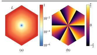
FIG. 5. Hexagonal geometry with side lengths  $L = 6\xi$ , and an applied current winding  $\Phi_I = 6\pi$ . (a) The pair correlation  $\Psi$ , showing a single vortex at the center. (b) The phase  $\varphi$  of the pair correlation, demonstrating that it is a giant vortex with winding number n = +3.
