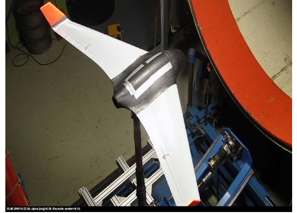
Fig. 2: The Skywalker X8 mounted in the wind tunnel
