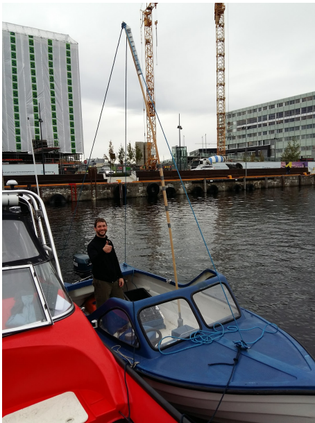
Figure 4. The 17 foot long target vessel, equipped with a radar reflector to improve radar visibility.
