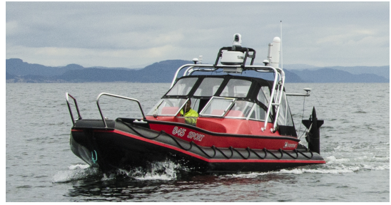
Figure 1. The Telemetron ASV, a dual-use vessel for both manned and unmanned operations. Courtesy of Maritime Robotics.
