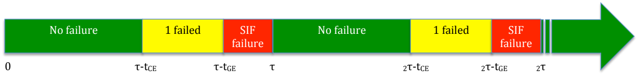
Figure 4.6: Failure development in a 1oo2 architecture
