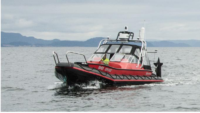
Fig. 1. The Telemetron is a dual-use surface vessel capable of operating as an ASV.
