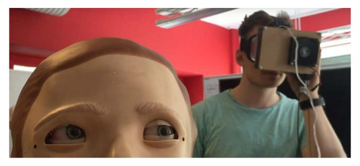
**Figure 1:** The operator (right) sees the live viewpoint of the mannequin (left) and directly controls the movement, incl. blinking, of the robotic eyes by the means of eye-tracking algorithms that are translated into according servo movements.
