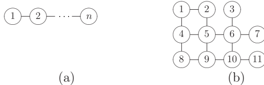
Figure 5: Two undirected graphs defining neighborhood systems. Two nodes are neighbors if and only if an edge is connecting them. A pairwise interaction, binary field which is Markov with respect to one of these neighborhood systems can be very efficiently handled by the exact algorithm described in Section 4.1. (a) A chain graph and (b) a somewhat more complex graph.
