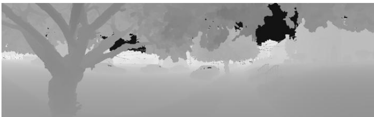
Figure 2.21: A range image showing a street scene in a residential area. The image is retrieved from the Brown database [Bro].
