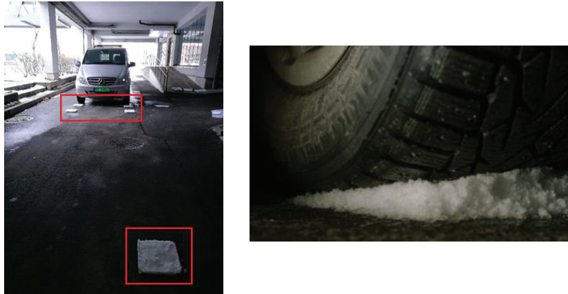
Figure 12 Placement of snow sample (marked in red) prior to testing
