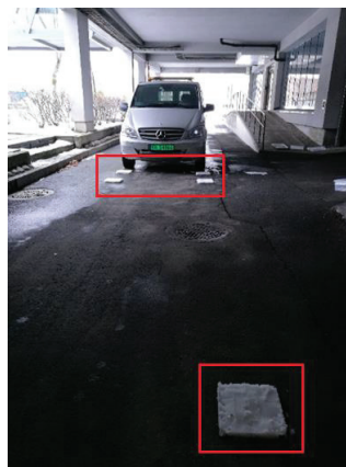
Figure 1. Placement of snow sample (marked in red) prior to testing.
