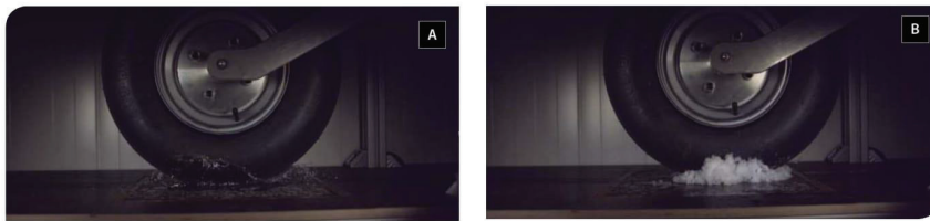
Illustration 2 - Tire Pavement Interaction in water and snow condition
