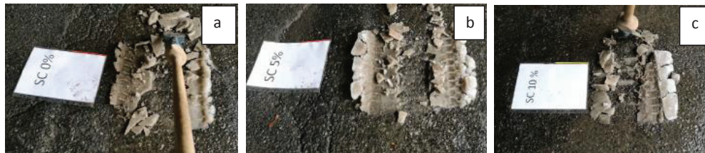
Figure 19 Showing snow having solution contents of 0.5 and 10 wt.% respectively after a scraping test. The snow, at 0 and 5 wt.% solution contents detached from the pavement in flakes, as can be seen in images 3 a) and b)
