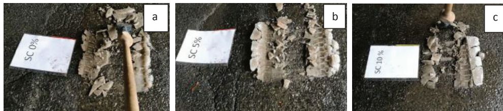
Figure 3. Showing snow with solution contents of 0,5 and 10 wt.% respectively after a scraping test. The snow, for 0 and 5 wt.% solution contents detached from the pavement in flakes, as can be seen in image 3 a) and b).
