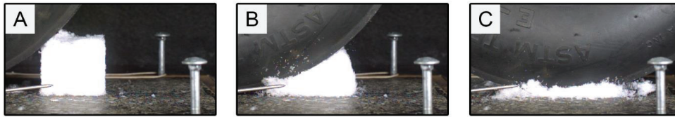
Figure 10 Snow sample before the test (a), during compression (b), after compression (c)
