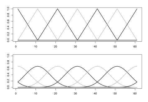
Figure 1.4: Uniform basis splines with degree one and three, in the upper and lower panel, respectively.
