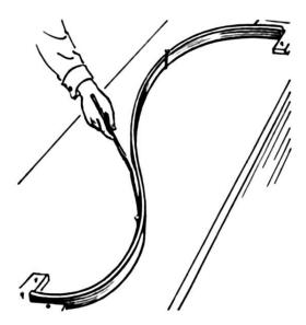
Figure 1.1: A flexible drawing device; the spline.
