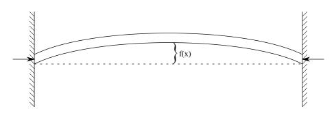
Figure 1.2: A bending rod deviating from neutral position.
