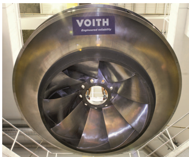
FIGURE 1. The runner of a 240-MW reversible Francis pump–turbine in the Limberg II pumped-storage plant, Austria. (Used with permission from [4].)
