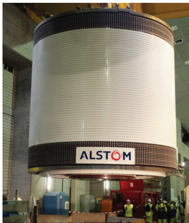
FIGURE 6. A motor-generator rotor of a 250-MW DFIM in the Linthal pumped-storage plant, Switzerland. (Used with permission from [61].)
