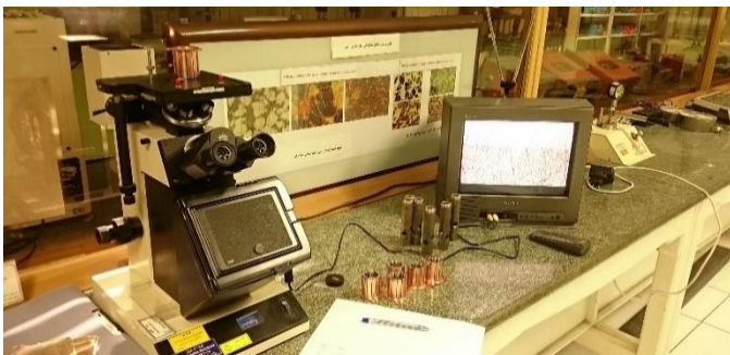
Fig. 2. Metallographic microscope with magnifications in the range of 100 to 800
