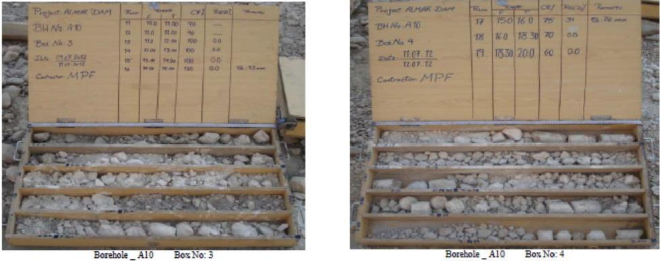
Figure 11: Borehole-A10, core samples at depth of 11-20 meters below the dam contact with foundation
