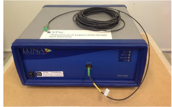
(b) The interrogator apparatus, LUNA OBR 4600
