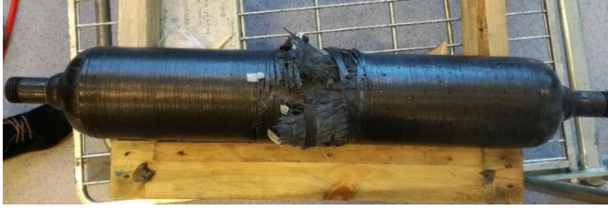
Figure 1: Pressure vessels before and after burst testing.
