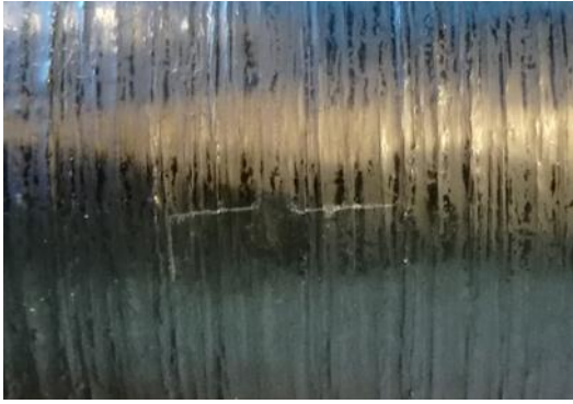
Figure 18: Severe impact damage on the cylinder surface
