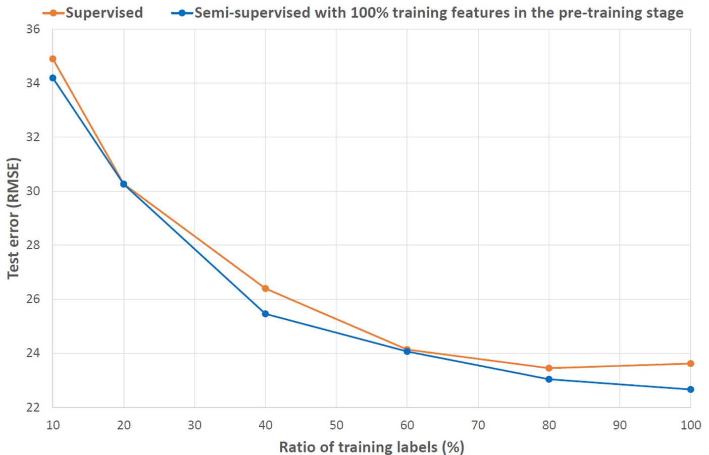
Fig. 5. RMSE comparison on subset FD004 when the labeled training data is reduced from 100% to 10%.
