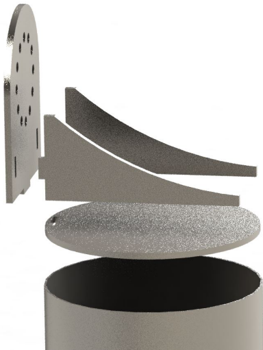
FIGURE 2. End plate on a link.
