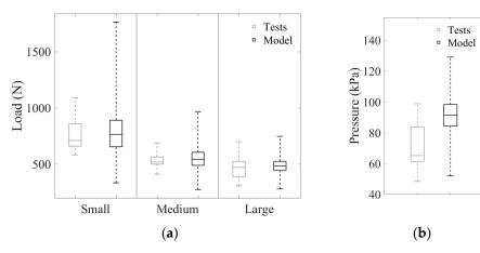
Figure 3. Failure load determined by laboratory tests and the strength prediction model in (a) fourpoint bending tests and (b) quasi-static pressure tests.
