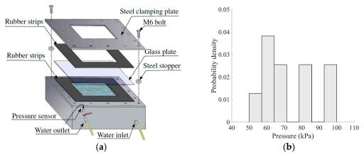
Figure 2. Quasi-static pressure tests: (a) assembly of the test set-up and (b) applied pressures at failure.
