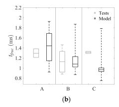
**Figure 4.** Time of fracture initiation  $t_{frac}$  in shock tube tests for group A, B and C determined by experiments and the strength prediction model, with  $K_{IC}$  set to (a) 0.75 MPa $\sqrt{m}$  and (b) 0.86 MPa $\sqrt{m}$  in the model.
