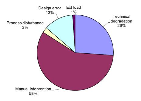
Figure 2 Overview of immediate causes of leaks (>0.1 kg/s), NCS, 2008–2015 (n=88)
