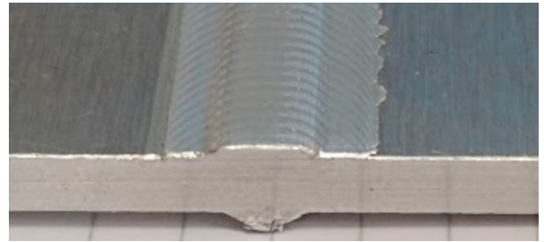
Fig. 3. Example of a HYB butt weld. The separate die at the rear of the stationary housing makes it possible to control the shape of the weld face.
