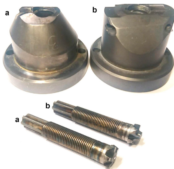
Fig. 5. Photograph of the tool parts used to build the layered structure; (a) pin and stationary housing used for stringer bead deposition; (b) pin and stationary housing used to fill the groove between the stringer beads.
