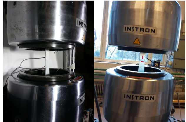
Figure 4: Placement and failure of the specimen in the test machine.
