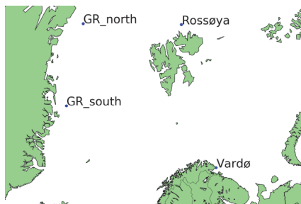
Figure 4. Placement of ground nodes in the Arctic region. Sensor Nodes: GR_north ( 80^\circ 52' 39.0''\text{N} 11^\circ 59' 53.0''\text{W} ), GR_south ( 75^\circ 51' 0.0''\text{N} 16^\circ 52' 15.5''\text{W} ) and Rossøya ( 80^\circ 49' 40.8''\text{N} 20^\circ 21' 0.0''\text{E} ). Ground Station: Vardø ( 70^\circ 22' 12.0''\text{N} 31^\circ 6' 36.0''\text{E} ).
