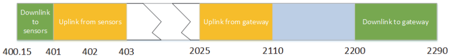
Figure 6.1: Possible frequency allocations for an EESS-service. Values are MHz. Green sections indicate downlink, yellow sections indicate uplink.
