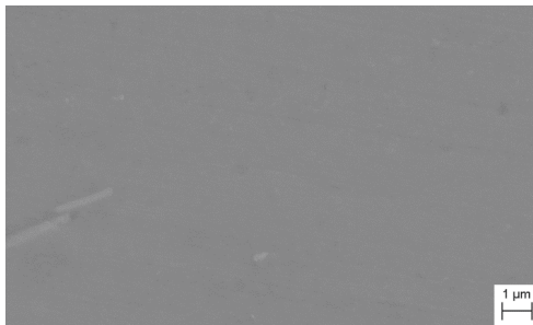
Figure 19. 6063 alloy showing a surface with no visible oxidation after exposure in 5CO 2 /95Ar for 90 min at 500°C.
