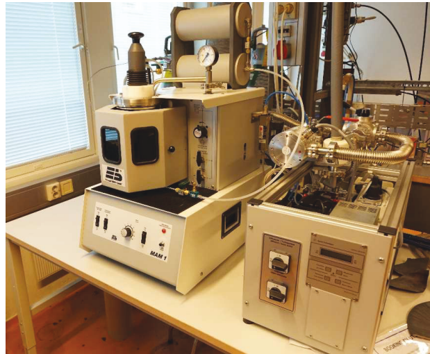
Figure 3-2 Arc-melter used to make master alloys.
