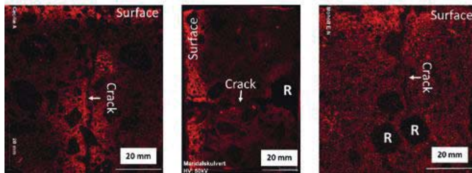
Figure 3 - \mu -XRF chlorine maps of concrete cores from de-iced structures. Left: Core C_0.45D from the Cecilie Bridge; Middle: Core T_0.45D from the Tåsen Tunnel; Right: Core M_0.55D from the Moholt Bridge. The orientation of the cores represents the surface orientation in the field. R = reinforcement
