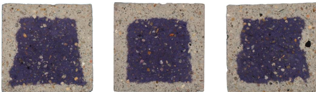
Figure 5: Carbonation detection in the plain A' (40x40x160 mm) mortar samples. From left to right: cross sections of A'-J, A'-V and A'-T. The samples were sprayed with thymolphthalein after 8 weeks of exposure.
