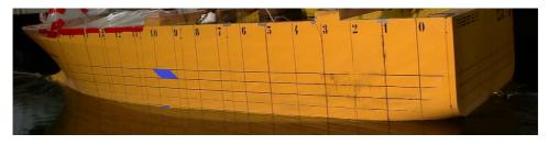
Figure 6.48: Sinkage and trim of the model in test C551.
