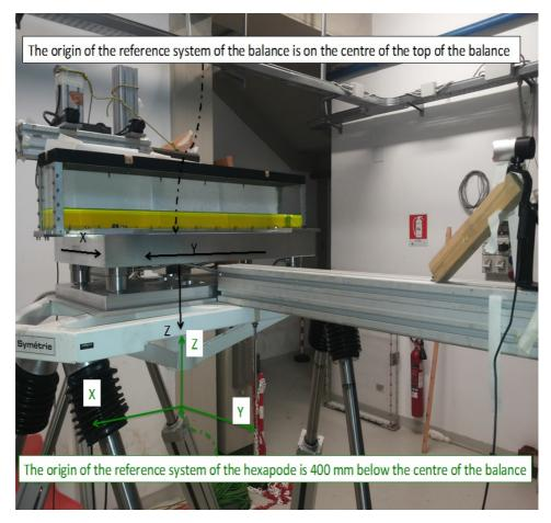
Figure 3.7: Sloshing tank and experiment set-up for isolated sloshing tests in CNR-INSEAN, Rome, Italy.
