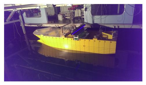
Figure 4.4: The ship model and the mounted free-surface anti-roll tank.
