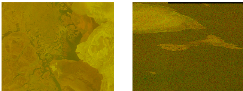
Figure 3.19: Sample GRD image used for sea ice extraction. Red = HH ; Green = HV
