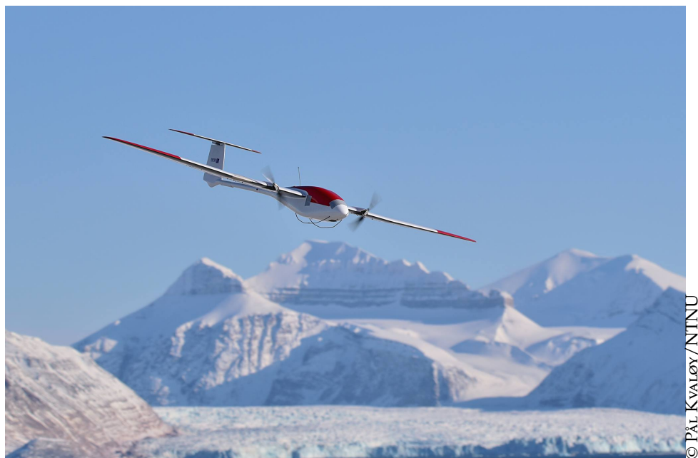
Figure 3.13: The CryoWing Scout, developed by Norut was flown to collect imagery of sea ice in Kongsfjorden
