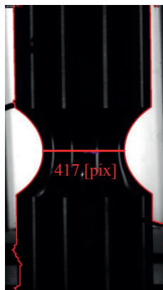
Fig. 6 Specimen image edges in Fig. 5 (a) derived with the edge tracing method. The minimum cross-section diameter is also shown in pixels.
