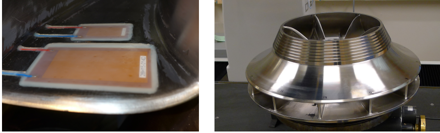
Figure 3: Left: Pads glued into the vane, Right: Runner ready for geometry measurement
