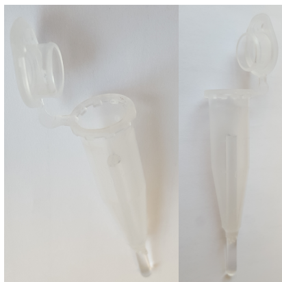
Figure 1: Image of Eppendorf tube with glass rod inside used for photopolymerizing pre-gel in squalane-PI.
