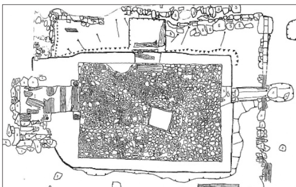
Figure 5.25. Stone cellar with cobbled floor, sump, external entrance with wooden stairs (left), trapdoor entrance (mid upper) and light well (right). The first provisioning managers' residence, Kongsgården (TA1991/1). After Nordeide 2000a: plan 25.
