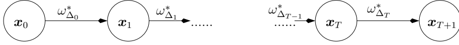
Figure 7: The figure shows the Directed Acyclic Graph (DAG) of the approximate fluid flow simulator. Thin arrows imply that there is a stochastic relationship.
