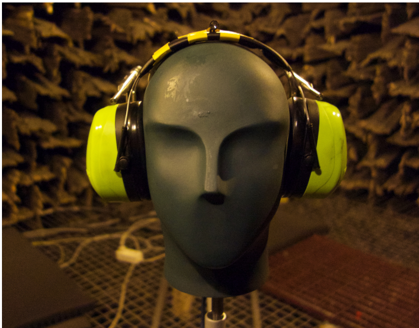
Figure B.7: Default test setup, microphones placed above each ear muff. Ultrasonic transmitter placed on top of head.
