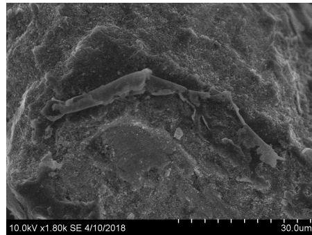
Figure 4.6: SEM micrograph of the surface morphology of the reacted contact mass from the P5 sample, extracted after 51 hours after termination, taken at a voltage of 10kV and current of 7A.
