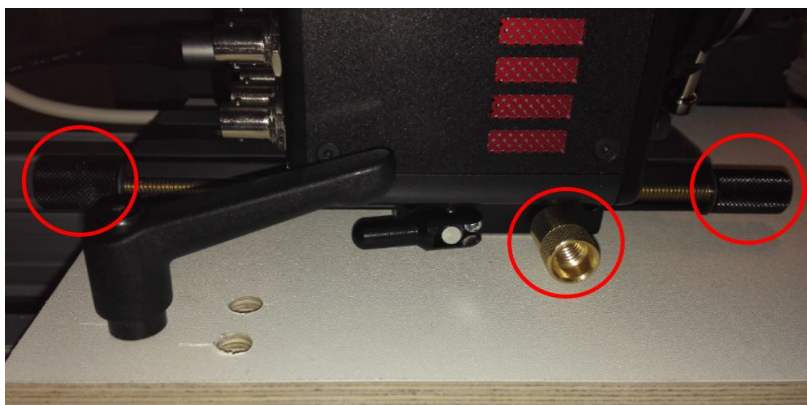
Figure 3.14: Mechanism for adjusting camera position
