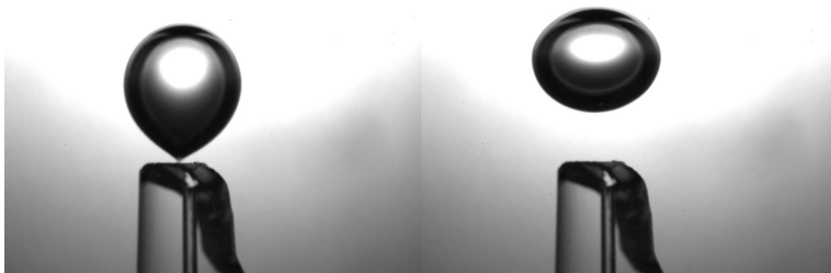
Figure 6.2: Bubble injection with glass needle
