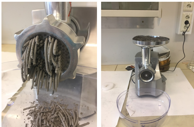
Figure 4.3: (left) Extrusion with calcined dolomite and cement Fondu through a dye with 3mm holes, (right) Kenwood Pro 2000 Excel Electric Mincer MG700.
