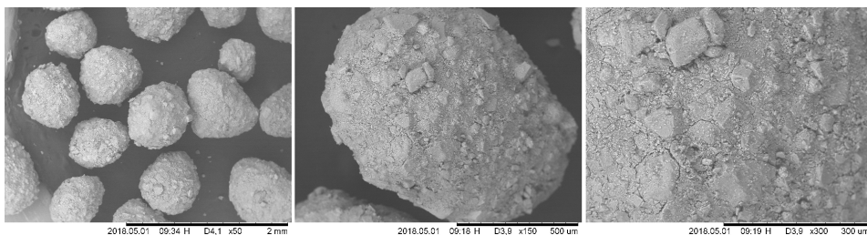
Figure A7.45: NO-10 SEM pictures of calcined pellets. (left) magnification x50 (middle) magnification x150 (right) magnification x300
