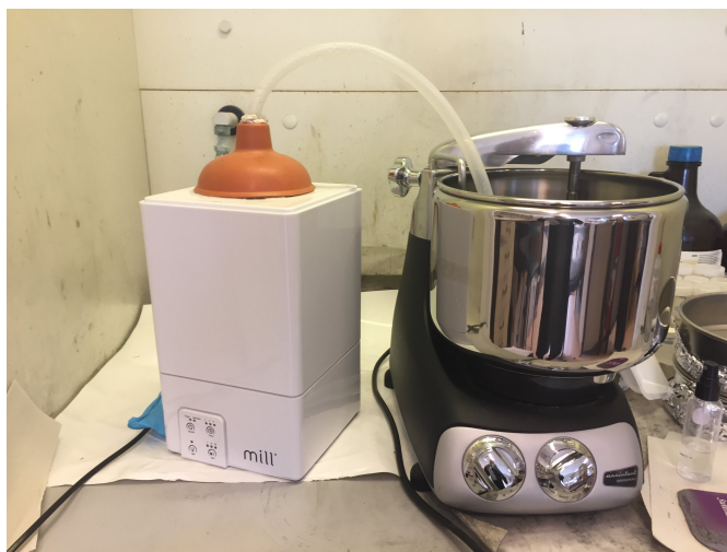
Figure 4.2: Rotary drum kitchen machine used as Granulator/Mixer. Equipped with humidifier to maintain near constant humidity in the bowl.
