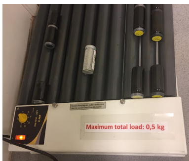
Figure 4.6: Ball miller (Cat) roller (RM10W-30V Cat) machine.
