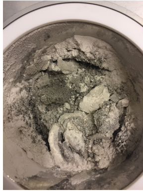
Figure A7.65: A figure of one of the experiments indicating bad stirring of water, dolomite and cement. The light grey material is dry dolomite/cement while the dark gray dolomite/cement is mixed with water.
