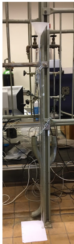
Figure 4.7: A 1.5m long glass tube used to simulate the fall of pellets in MBCL
