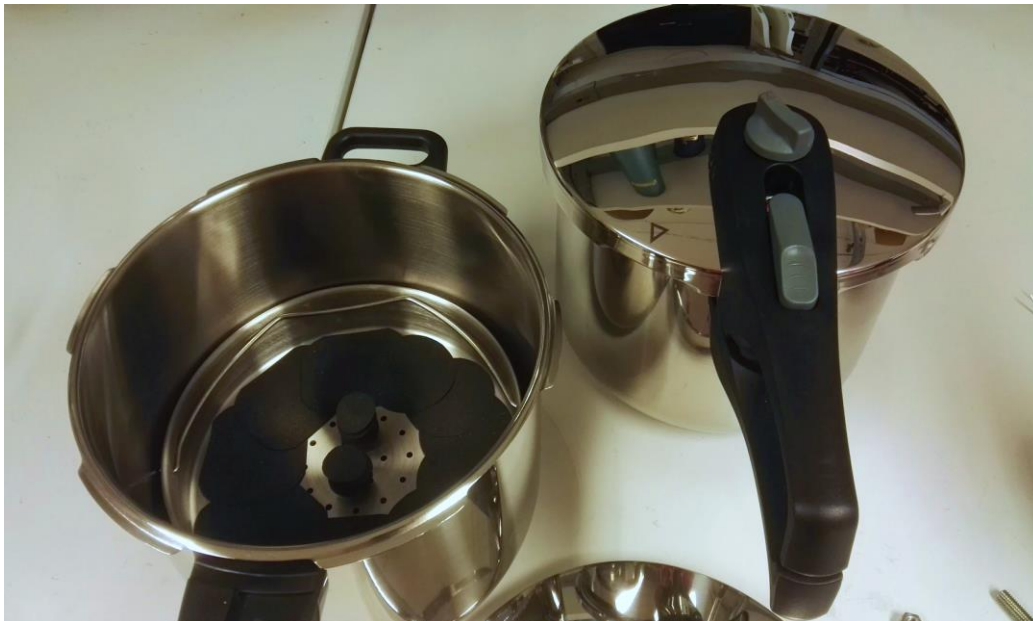
Figure 17. Samples placed in pressure cookers during ageing
