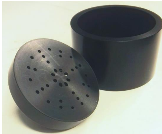
Figure 16. Cup and piston apparatus for swelling height measurements
