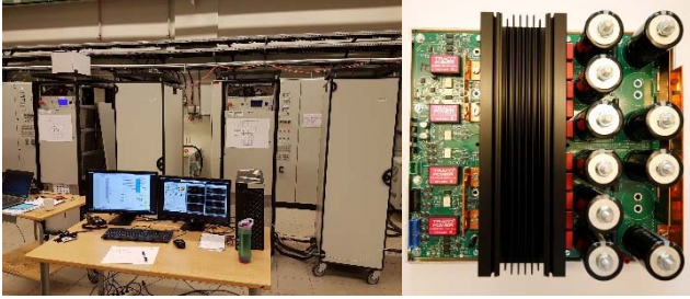
Fig. 3. Overview of laboratory setup and picture of circuit board with two half-bridge sub-modules
