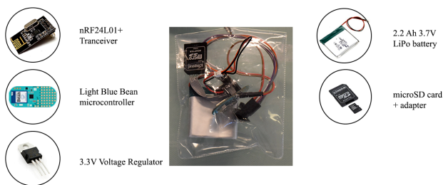
Fig. 1. Parts of an active RF transceiver prototype [9].
