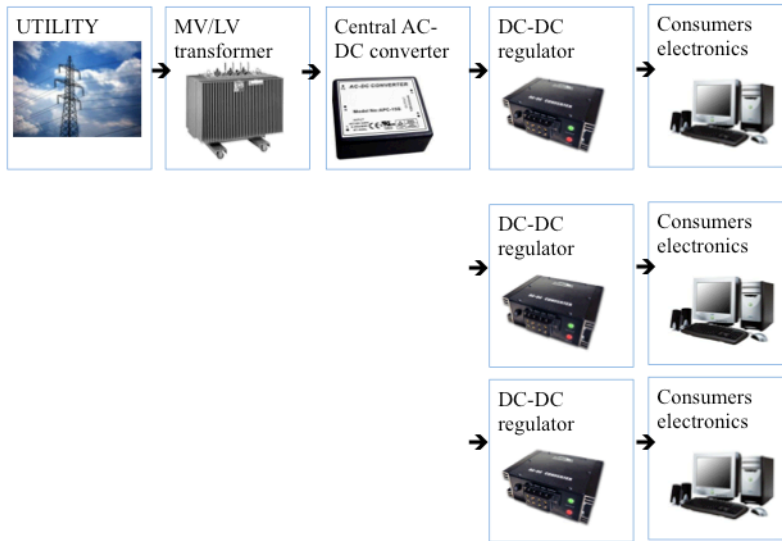
Figure 6: Schematic illustration of the proposed DC system solution [43]-[46].
