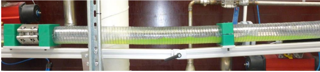
Figure 24: Liquid accumulated in the bottom of the dip when the gas flow was choked.
