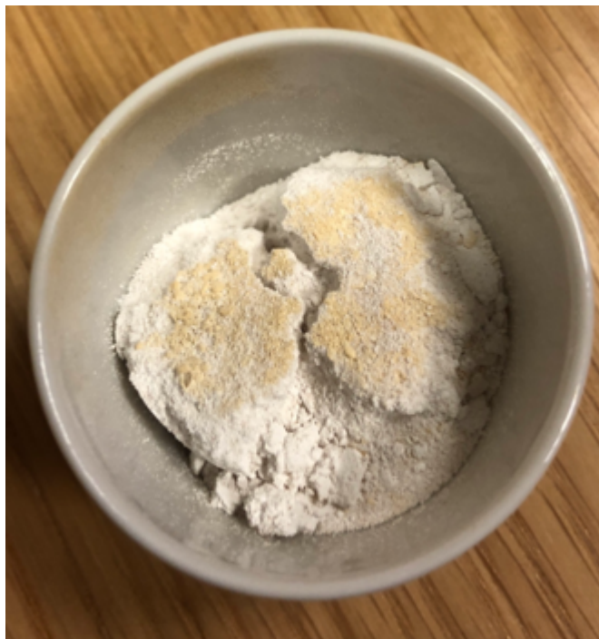
Figure 4.3: shows a picture taken of B3 after being calcined in the high-temperature furnace. Observe the color of the top layer.
