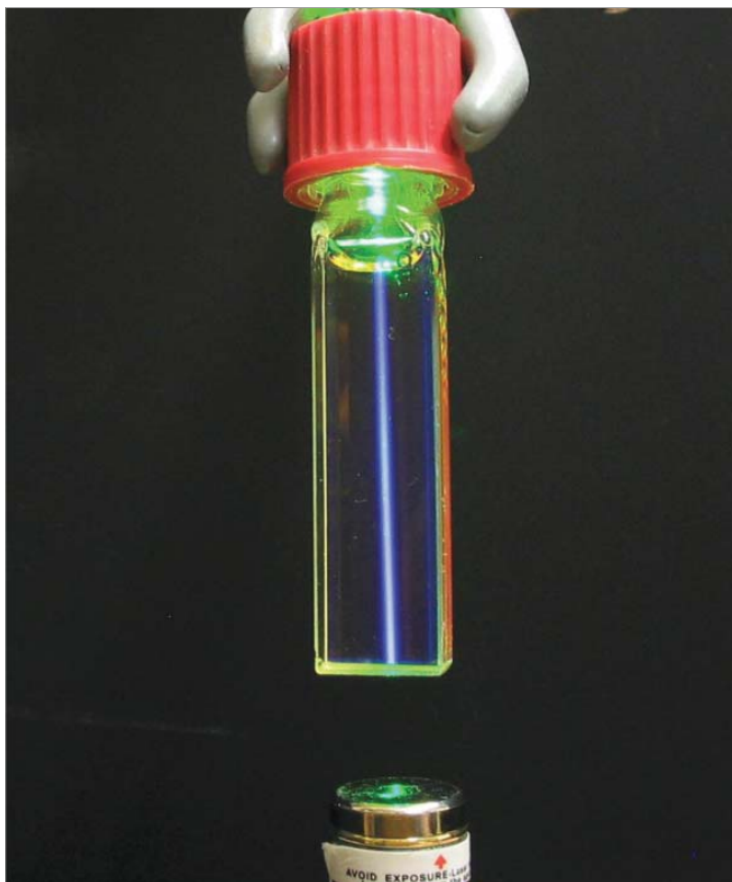
Figure 2.10: Shows a green laser shining on a solution, containing ruthenium(II) complex and a 9,10-dphenylanthracene, that is upconverting green photons to blue photons. Reproduced from [40]
