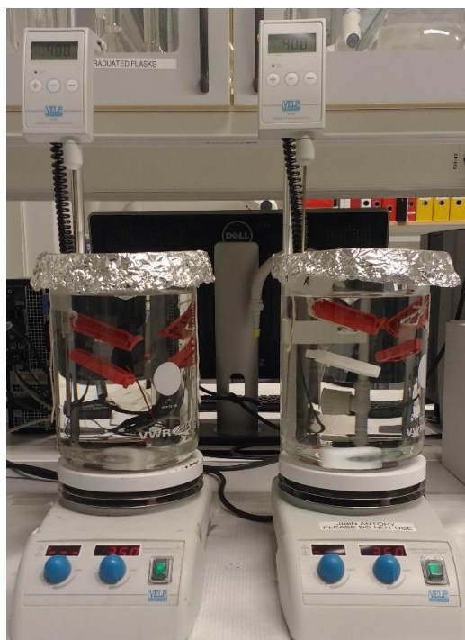
Figure 3.12: Samples kept on dialysis at release conditions.
