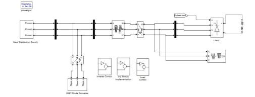
Figure 9.2: Simulink model of the system with ideal power supply and non-linear load
