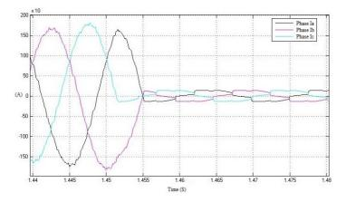
Figure 6.12: Three phase source current with and withou connecting the VFDs
