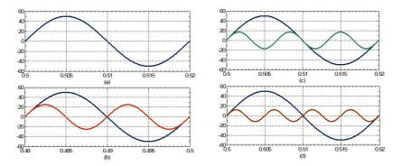
**Figure 4.6:** Comparison of Harmonic and fundamental components of the voltage (a)fundamental component (b) second harmonic with fundamental component (c) third harmonic and fundamental component (d) fourth harmonic and fundamental component
