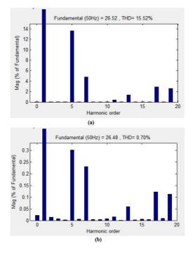
**Figure 6.7:** (a) FFT analysis before connecting the converter (b)FFT analysis after connecting the converter
