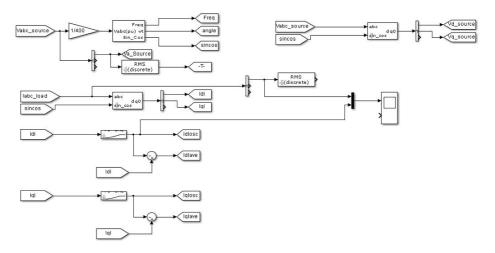
Figure 9.8: Block diagram of implementation of Clark and Park Theory
