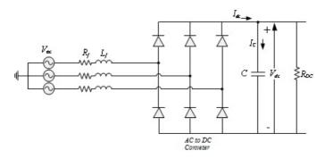
Figure 5.2: Three phase diode bridge rectifier
