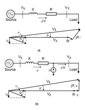
Figure 9.20: (a) The system with no compensation (b) The system with shunt compensation [14]
