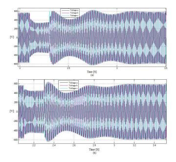
Figure 6.15: (a) Three phase to ground fault with no reactive power compensation (b)Three phase to ground fault with reactive power compensation by one VFD  $% \left( {{\rm VFD}} \right)$
