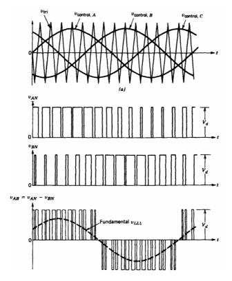
Figure 3.10: Three phase inverter waveform with PWM [49]
