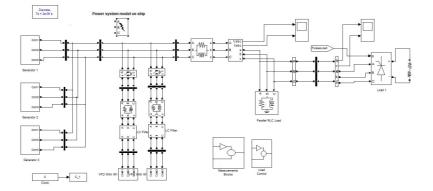
Figure 9.4: Power system on ship with parallel operating generators, two VFDs and non-linear load
