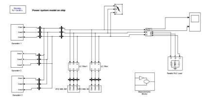
Figure 9.6: Power system on ship with parallel operating generators, two VFDs for reactive power control
