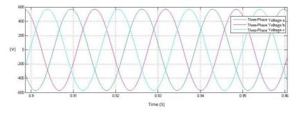
Figure 6.3: Bus bar voltages without connecting the VFD
