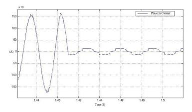
Figure 6.13: Single phase source current with and without connecting the VFDs
