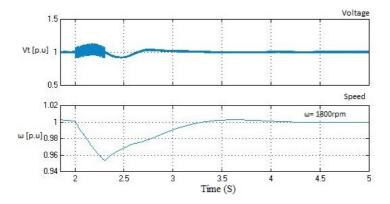
Figure 9.18: The impact of three phase to ground fault on SG parameters
