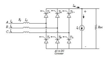
Figure 5.3: Three phase thyristor bridge rectifier
