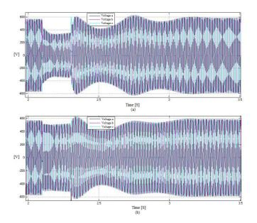
**Figure 6.17:** (a) Three phase to ground fault with no reactive power compensation (b)Three phase to ground fault with reactive power compensation by two VFDs
