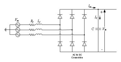
Figure 3.7: Three phase diode rectifier
