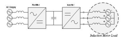
Figure 5.4: Variable frequecy drive with IGBT rectifier and inverter
