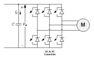
Figure 3.9: Circuit diagram of three phase inverter
