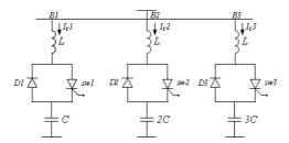
Figure 9.23: Thyristor-diode switched capacitor compensation [29]
