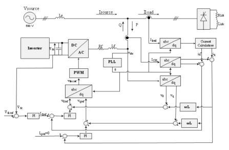
Figure 5.7: Control of VSC rectifier [27]
