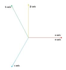
**Figure 5.9:** Three phase and  $\alpha - \beta$  coordinates [44]
