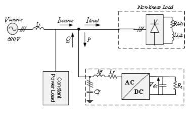
Figure 6.4: Power system with ideal supply and non-linear load
