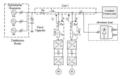
Figure 5.1: General figure of the power system of ship
