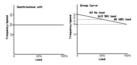
Figure 3.3: Typical figures of Isochronous unit and 5% Droop curve [52]
