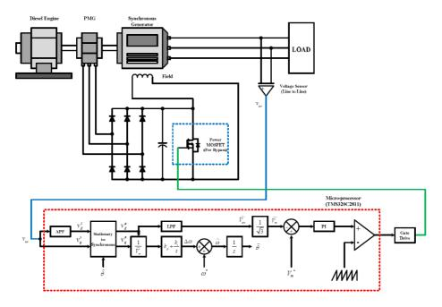
Figure 3.5: Complete block diagram excitation control of ship SG [31]
