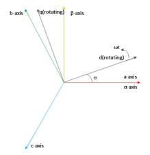
**Figure 5.10:** Three phase coordinate system,  $\alpha - \beta$  coordinates and *d-q* coordinated systems. [44]
