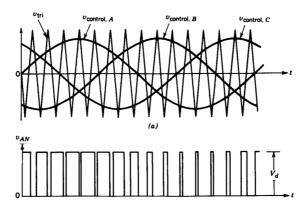
Figure 5.17: Pulse width modulation waveform [49]
