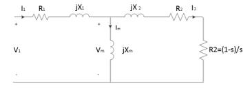
Figure 3.11: Induction motor equivalent circuit
