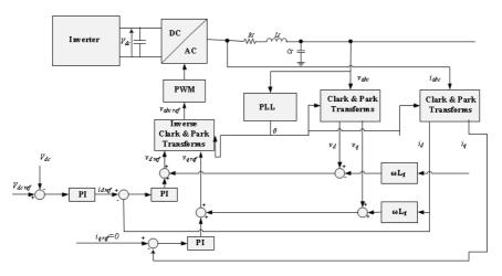
Figure 5.8: Use of Clark and Part transformation in the control of rectifier
