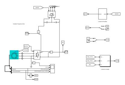
Figure 9.7: Block diagram of VFD with induction motor as load
