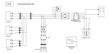
Figure 9.5: Power system on ship with parallel operating generators, one VFD for reactive power control
