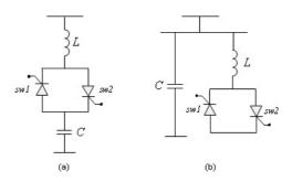
Figure 9.22: (a) Thyristor controlled capacitor circuit (b) Thyristor controlled reactor cicuit [29]
