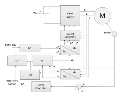
Figure 5.16: Control scheme for inverter of variable frequency drive
