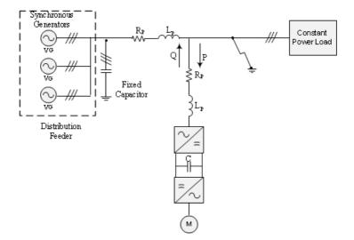
Figure 6.14: The power system with one VFD installed
