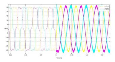
Figure 6.5: Three phase source current before and after connecting the converter
