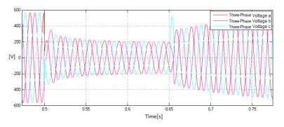
Figure 4.2: The voltage dip in case of three phase to ground fault
