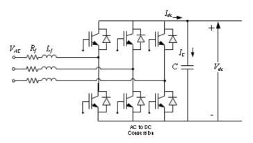
Figure 5.5: Circuit diagram of IGBT based rectifier used in the VFD
