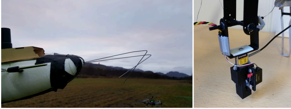
Figure 11: Left: Metallic hooks attached to the nose of the fixed-wing UAV, used to latch onto the suspended net. The hooks had little to no effect on flight performance. Right: Assembled quick-release mechanism and tension sensor on a gimbal-like structure for free range of motion.
