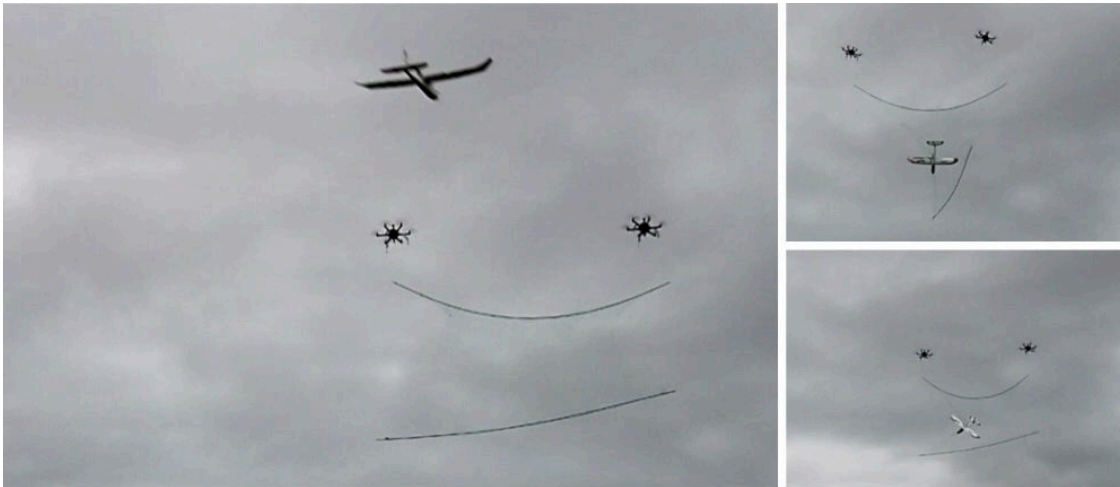
Figure 1: Image from the experimental validation. The fixed-wing UAV is approaching the net, which is being carried by two multirotor UAVs. On the right, the fixed-wing UAV is arrested by the net, and stays attached due to hooks on the nose of the UAV.
