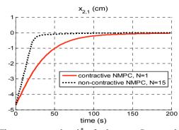
Fig. 9. The state  $x_{2,1} = h_2 - h_2^*$  of subsystem S<sub>2</sub> - case b).
