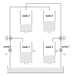
Fig. 1. Quadruple-tank system (Johansson (2000)).
