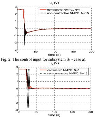
Fig. 3. The control input for subsystem  $S_2$  - case a).
