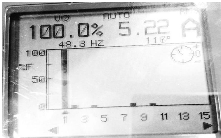
Figure 73: Voltage harmonics with U_{st} = 0.34 , f_s = 48.3 Hz
