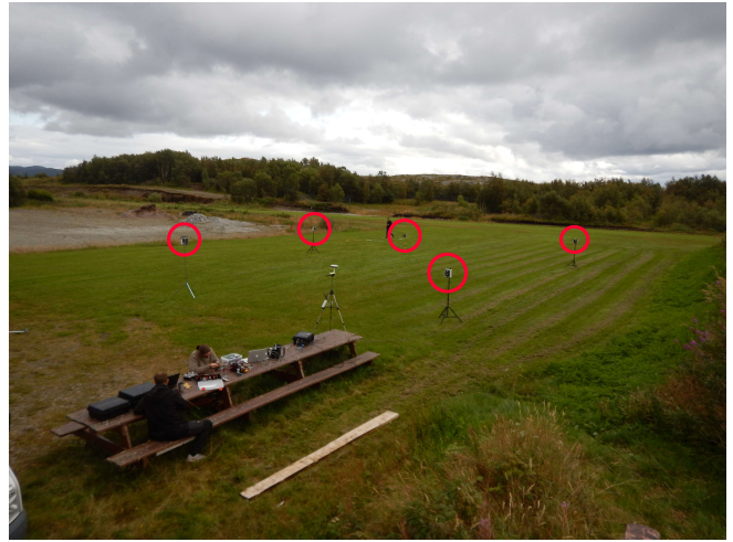
Figure 6. Typical UWB anchors constellation setup during flight tests
