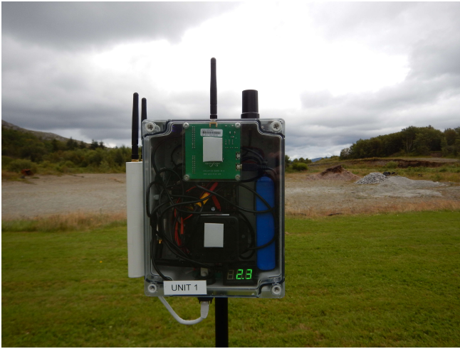
Figure 5. UWB anchor used during flight tests.
