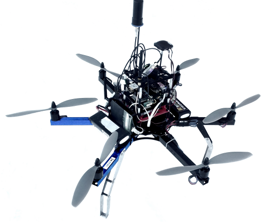
Figure 4. Multirotor UAV with GNSS RTK and UWB systems on board.
