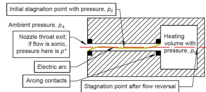
Fig. 1 An arcing chamber connected to a heating volume (schematic). The drawing is axisymmetric along the horizontal center axis and the electrodes are ring contacts.
