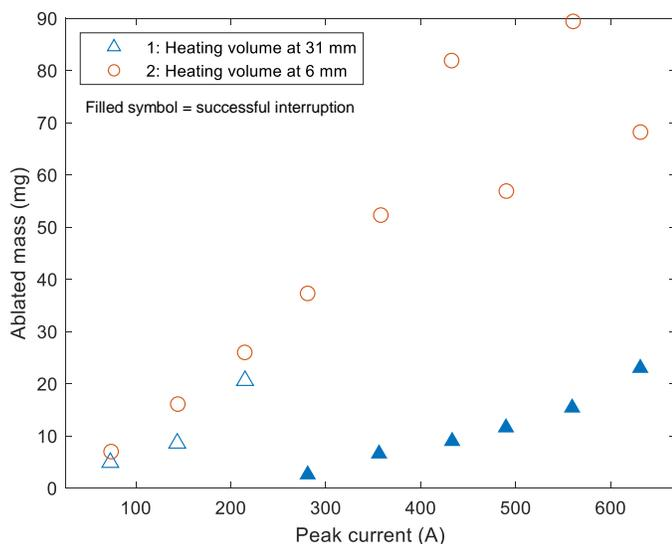
Fig. 8 Ablated mass from the nozzle at different current amplitudes. The ablation is significantly lower in the case of successful interruptions (filled symbols) with arcing time of about 10 ms. In failed interruptions (open symbols), the total arcing time is up to 50 ms, but varying because of varying reignition voltage.
