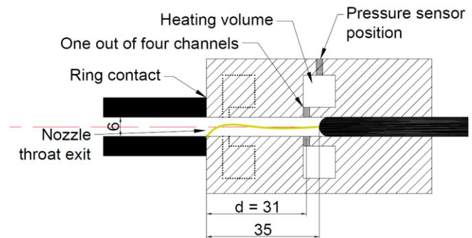
Fig. 2 Sketch of model switch 1, showing the volumes and pressure sensor position. The switch is axisymmetric around the center axis. The connecting channels (grey) are not axisymmetric. Details are given in Table 1. The heating volume position of switch 2 is indicated by dotted lines. Dimensions are in millimeters.
