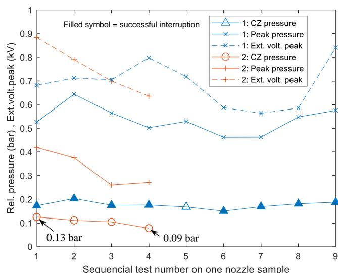
Fig. 9 Consecutive tests on one nozzle sample at a current of 240 A rms, showing the evolution in CZ blow pressure, peak pressure and extinction voltage peak in switch 1 and 2. Filled symbols indicate successful interruptions. The fifth test on switch 1 (in blue) resulted in a reignition after the first CZ, and successful interruption on the second CZ.
