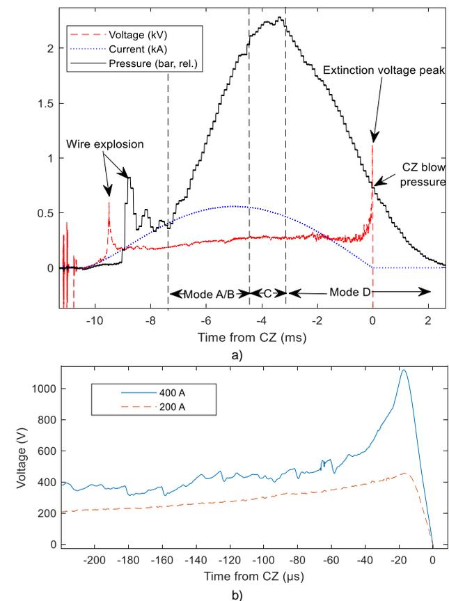
Fig. 5 a) Results from experiments with the heating volume at 31 mm from the nozzle throat exit (switch 1). The different flow modes, as described in Section II.B, are indicated. b) High resolution view of the extinction voltage peak at 400 A and 200 A.
