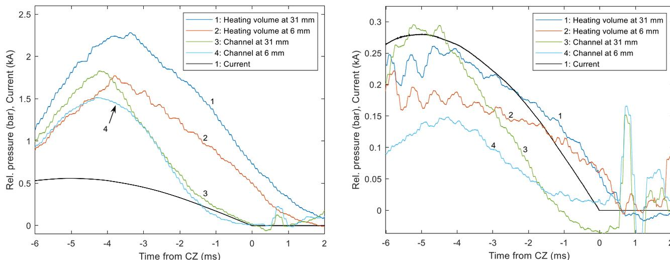
Fig. 6 Pressure evolution in the experiments at 400 A to the left and 200 A to the right. The black line shows the current waveform for the test with switch 1. Colored lines show the pressure in the heating volume in the four different switches. The pressure rise after CZ in switches 2-4 is due to re-ignitions. A possible explanation for the negative relative pressure values (under-pressure around CZ) is the contraction of the arc core as the current and temperature decrease.
