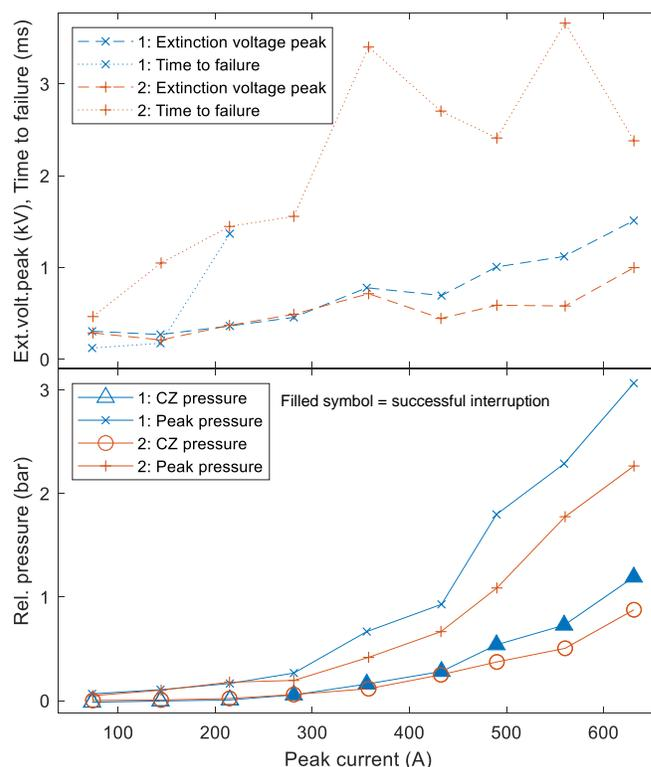
Fig. 7 Results for switch 1 and 2 at currents from 50 to 450 A. Only the first CZ is considered. CZ pressure and peak pressure are shown in the lower figure. Successful interruptions are indicated by filled symbols at the related CZ pressure. Extinction voltage peak and time from CZ to failure are shown in the upper figure.
