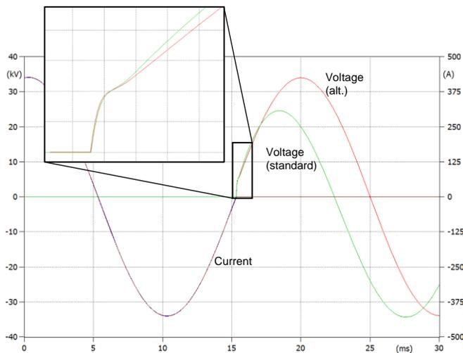
Fig. 4 Simulation results showing the current and voltage waveforms derived from the standard IEC 62271-103 (green) and with the alternative test circuit (red). The transient recovery voltage (TRV) is nearly identical up to 22 kV. After that, the TRV of the alternative circuit continues up to the peak of the source voltage, giving a more onerous duty.
