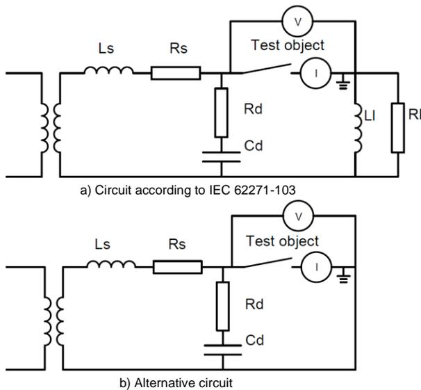
Fig. 3 Circuit diagrams according to the standard (a) and the alternative circuit (b) that, after adjusting the impedances, produce the same current and voltage up to a certain point. Voltage and current measurement sensors are indicated. Supply elements are denoted with  $s$ , load elements with  $l$ , and damping elements with  $d$ .
