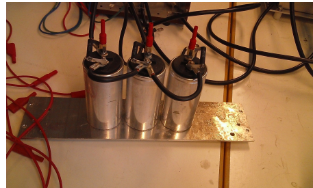
(b) Star connected three phase capacitors of the filter on the converter side.
