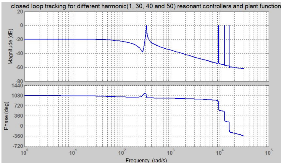
Figure 2.15: Reference tracking by the discretized current controller for h=1, 30, 40 and 50 .
