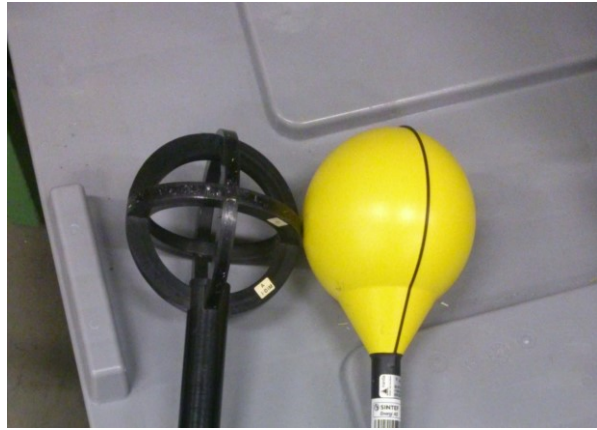
Figure 4.5 - Analog EMC field analyzer probe and Narda EMF-300 probe.
