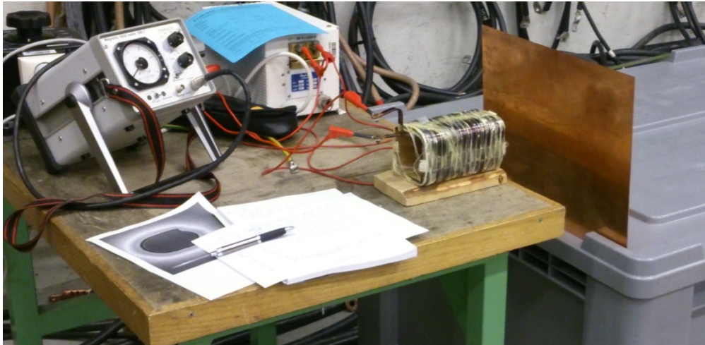
Figure 4.8 - Photo of test set-up with a copper plate in front of the coil to test the effect of electromagnetic shielding.
